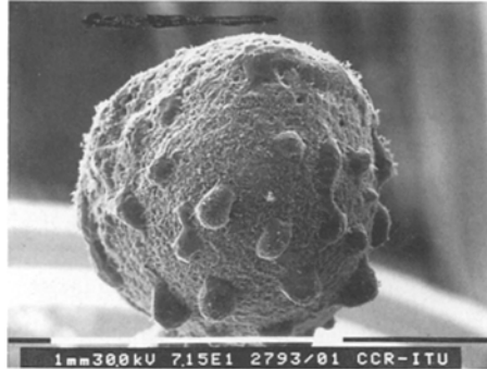
Fig. 2. RW graphite sample with droplets of frozen liquid (SEM micrograph).
